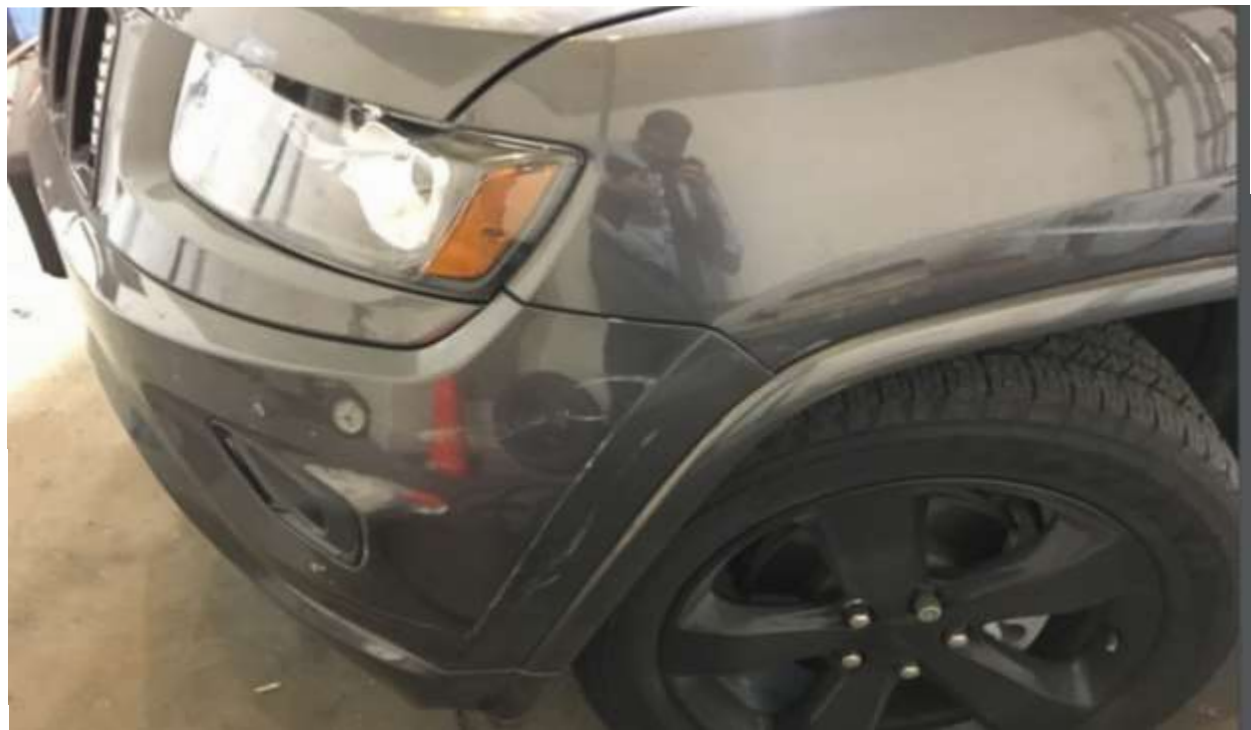
Figure 5. Photo showing minor impact damage to the front driver's side bumper of the Jeep. 31
