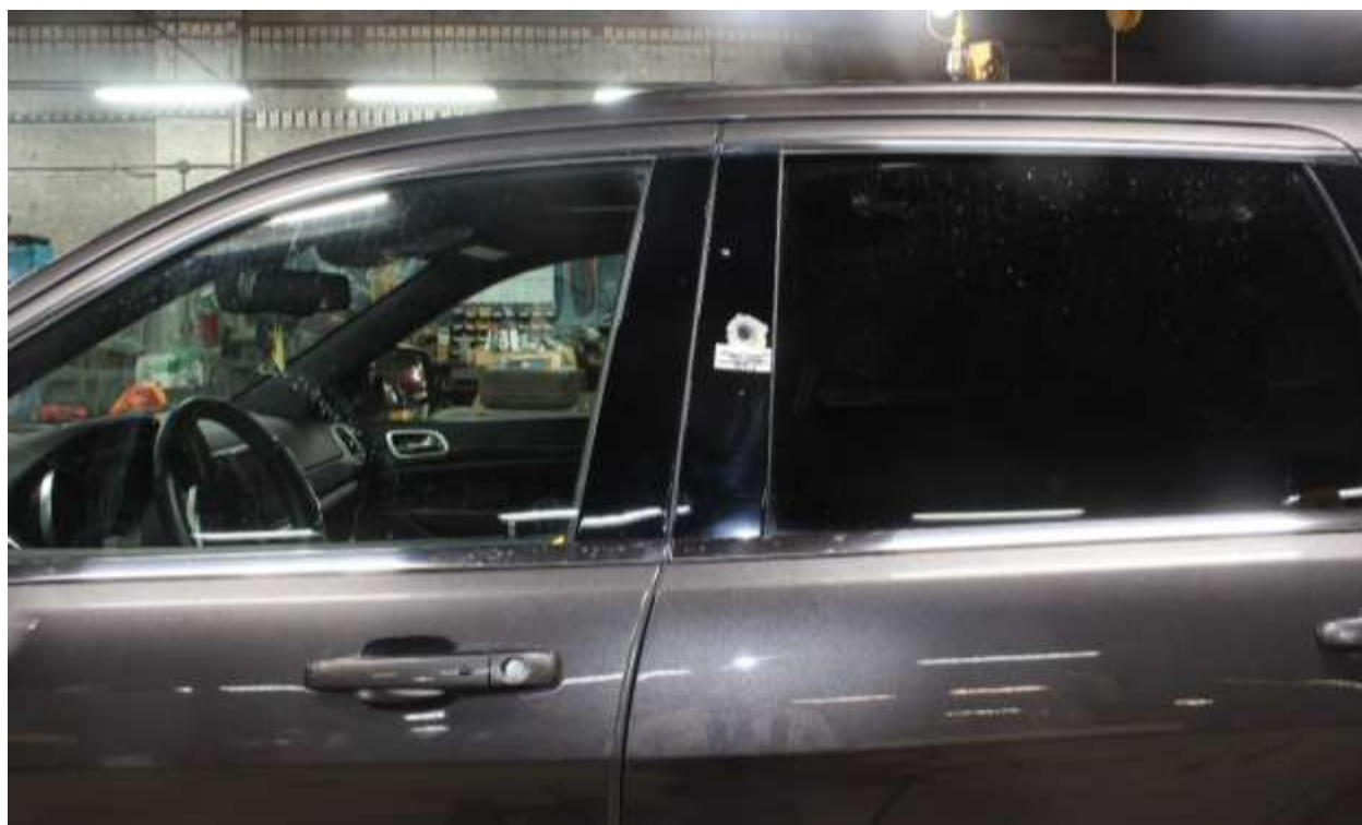
Figure 3. Photo showing apparent gunshot damage to the rear driver's side door pillar of the Jeep. 29
