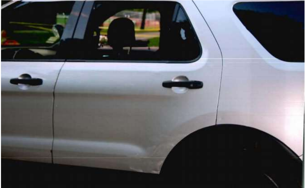
Figure 6. Photo showing minor impact damage to the rear driver's side door of the police SUV. 32
