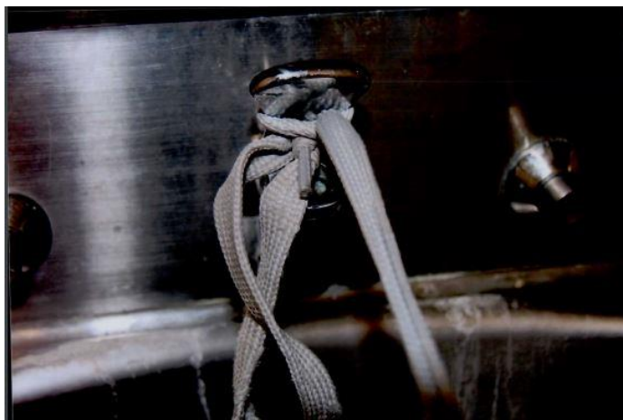
Figure 4. Close-up photograph of the draw-string attached to the faucet with aglet intact.
