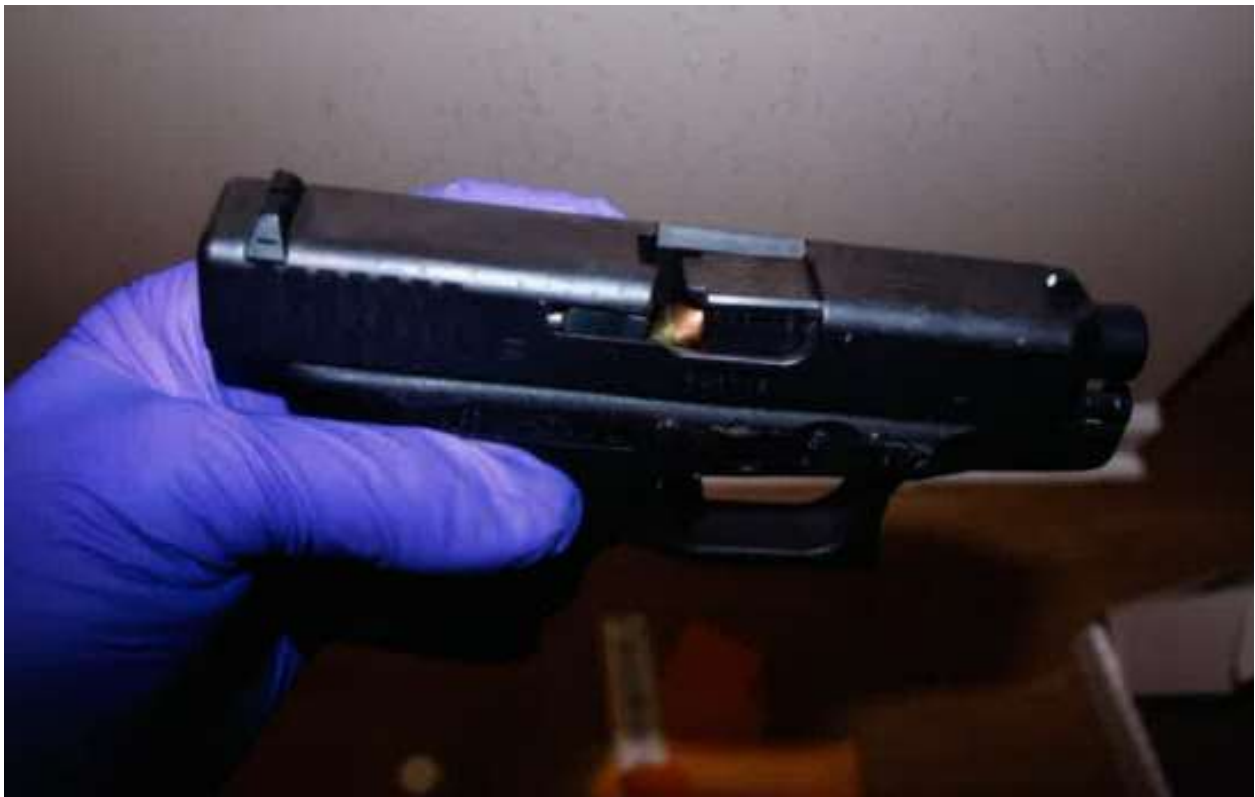
Figure 2. ET photo showing the Glock Model 26 pistol with a failure to feed malfunction.
